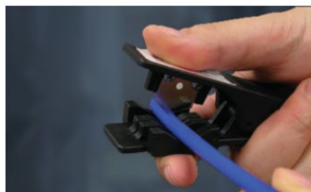
Cut the tube square and remove any burrs or score marks.
