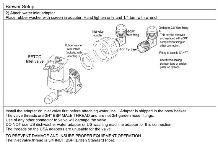
This valve is not a standard USA washing machine or dishwasher thread (3/4" GHT)
