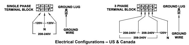
Finally, connect the incoming power wires to the terminal block in accordance with applicable codes.
