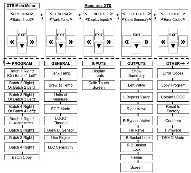
\*Single side brewer only shows the four RIGHT menus—dual brewers show LEFT and then RIGHT Batch 1—Right and Left are permanent-may not be deleted and are completely programmable †Batch 2-4—Right and Batch2-4—Left may be individually selected-or-entirely deleted
