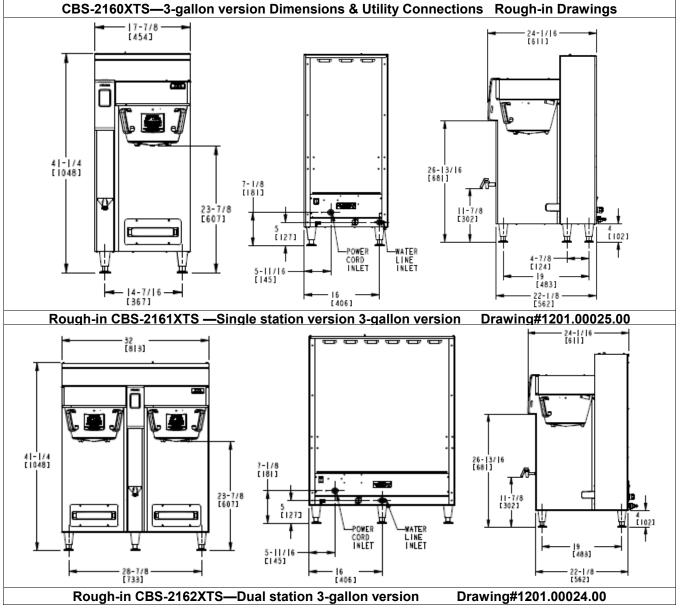
All brewers HARDWIRE to an internal TERMINAL BLOCK See wiring diagrams for connections
