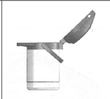
**2** Squeeze the **Lid Release Buttons** to release the lid.
