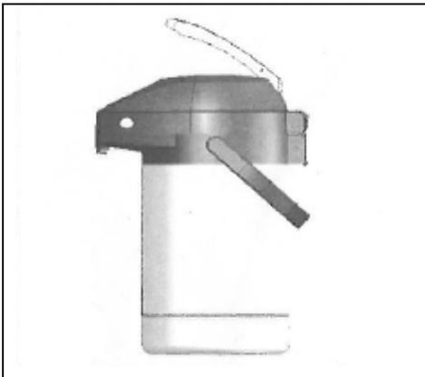
**4** Clean the interior of the tank with warm water, detergent and a brush. Proprietary airpot cleaners may also be used. **Do not put the airpot into an automatic dishwasher. Do not allow solutions containing chlorine to remain in tank.**
