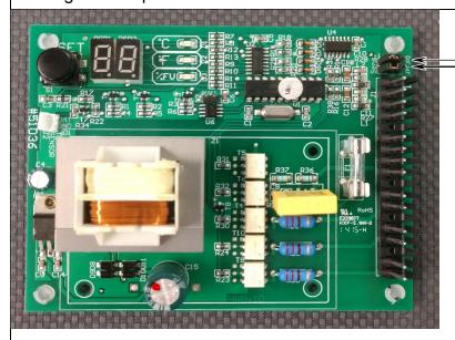
The HWB can be set to detect high purity water by moving the two bias jumpers [JP1&JP2] to "HI"
